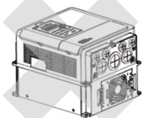
B. Horizontal installation
