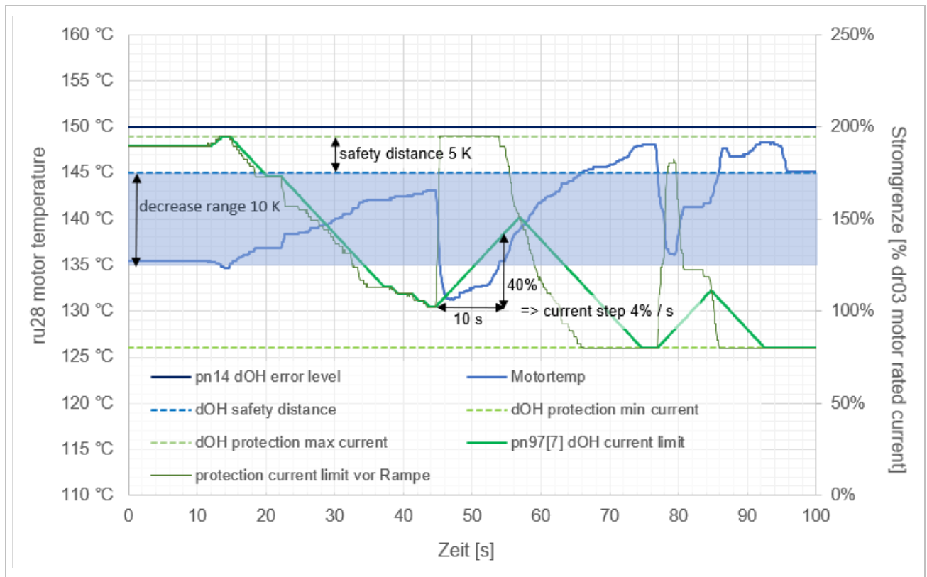
Figure 16: Graph of the current limit depending on the motor temperature
